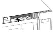
4. Lift the bottom of the charcoal filter. Slide the filter straight out.
