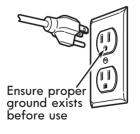
WARNING: Improper grounding can result in a risk of electric shock. Consult a qualified electrician or service technician if you do not understand the grounding instructions, or if you wonder whether the appliance is properly grounded. Do not use an extension cord. If the power supply
