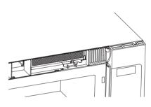
9. Reinstall the vent by sliding the bottom of the vent into place. Push the vent top into position and slide right until it snaps into place. Replace the two vent mounting screws located on top of the microwave using a #1Phillips screwdriver.
