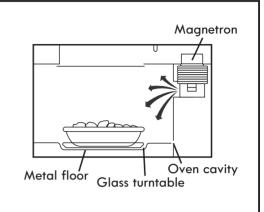
**Microwaves** pass through most glass, paper, and plastics without heating them, so food absorbs the energy. Microwaves bounce off metal containers so food does not absorb the energy.
